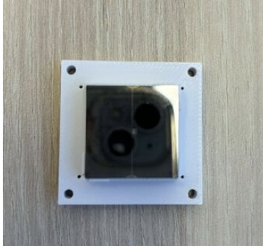
Figure 19: 3D printed part of the third design with the chip inserted into the slot.
